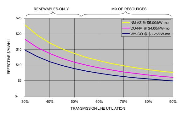
Projections were made for power delivered via HPX and compared against the projections for in-state resources (*Figure 8*). Subsidies currently available to the solar and wind industries<sup>11</sup> were not incorporated in the analysis, as those subsidies may change or be eliminated by HPX's proposed on-line date of 2017. In addition, the effect of varying "CO<sub>2</sub> tax" scenarios where modeled
