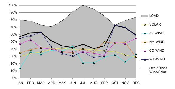
Figure 10: Monthly Wind & Solar Performance vs. Load Requirement
