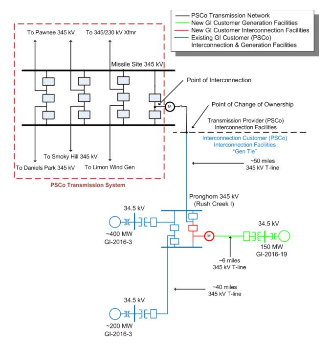
Figure 2: GI-2016-19 Interconnection to 345 kV Bus in Missile Site Substation
