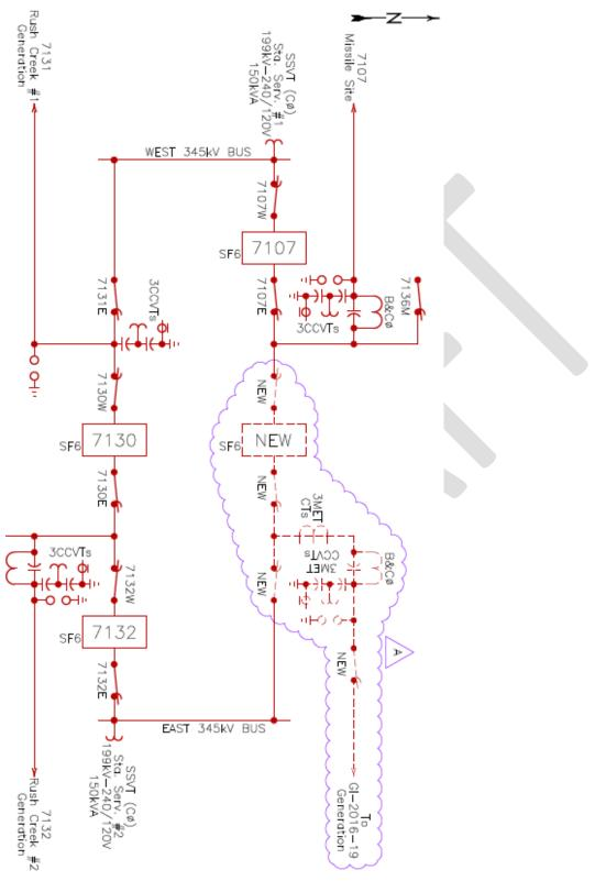
Figure 3: GI-2016-19 Physical Connection at Pronghorn Switching Station
