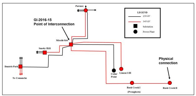
Figure 1: Missile Site and Surrounding Transmission System
