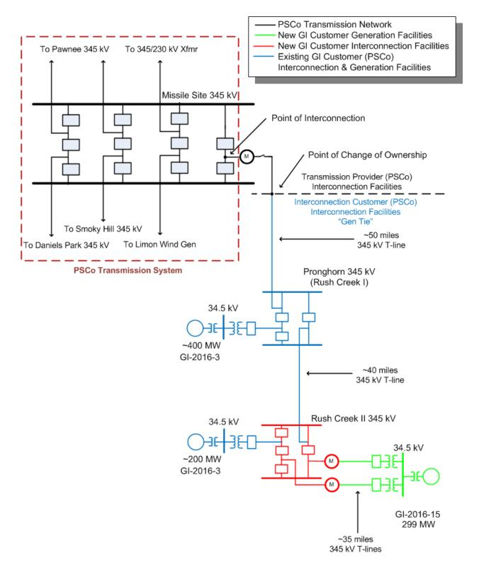
Figure 2: GI-2016-15 Interconnection to 345 kV Bus in Missile Site Substation (includes Pawnee-Daniels Park 345 kV project)
