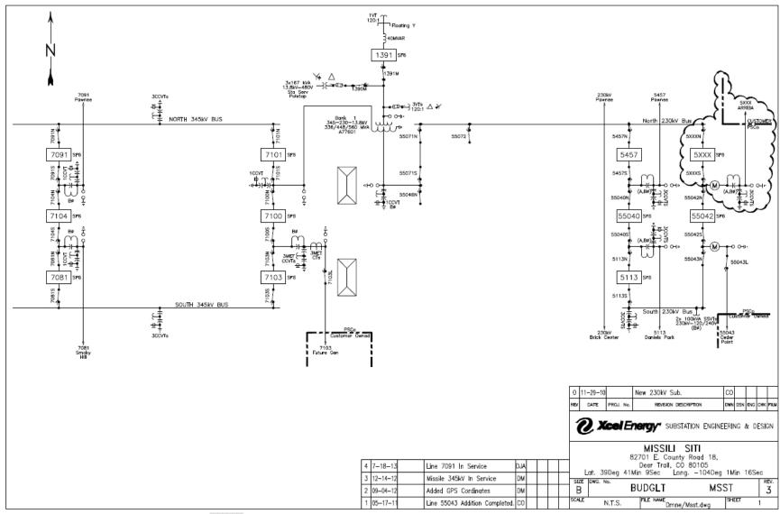
Figure 1 Missile Site Substation Interconnection
